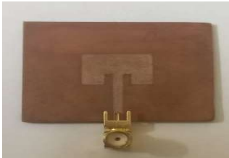
Figure12: Fabricated Single Patch Antenna
