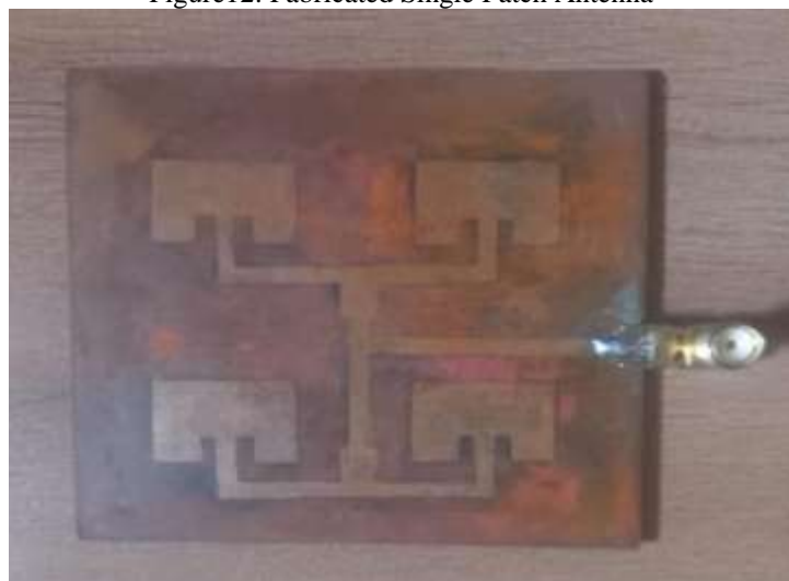
Figure 13: Fabricated 2x2 Microstrip patch Antenna Array
