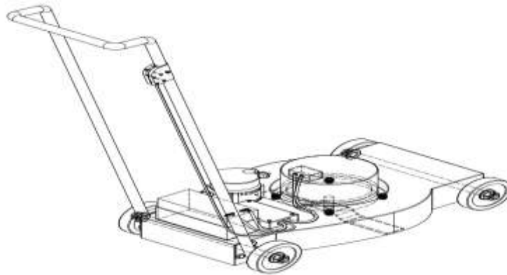
Figure 2. 3D Model of the Mower Deck and Engine
