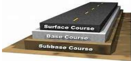
Figure 1: showing layers of flexible pavement
