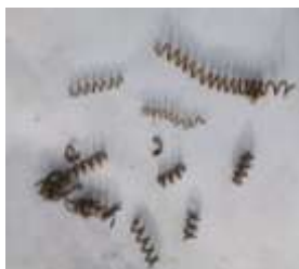
(a) Rusted and broken heating element (b) Rusted and broken heating element Plate 7 (a to b): Broken heating element after usage
