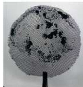
(a) Bio oil-stained sieve for 1 kg at 200 °C (b) Bio oil-stained sieve for 1 kg at 300 °C
