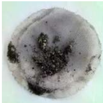
(c) Trapped biochar from 2 kg at 400 °C
