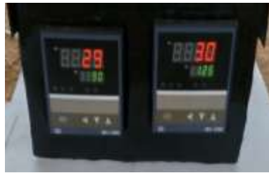
(c) Digital LCD Temperature indicator
