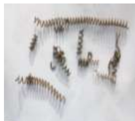
(a) Rusted and broken heating element (b) Rusted and broken heating element Plate 7 (a to b): Broken heating element after usage
