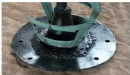
(a) Top flange for closing reactor
