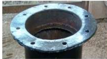
(b) Bottom flange for closing reactor
