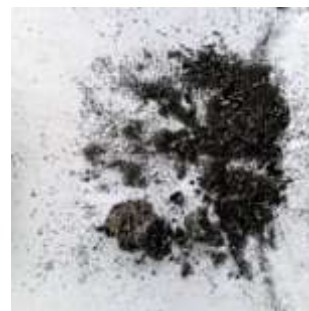
(b) Trapped biochar from 3 kg at 500 °C
