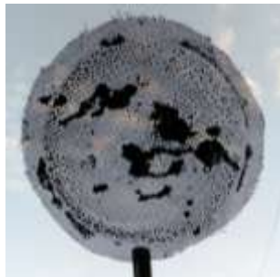
(c) Bio oil-stained sieve for 2 kg at 200 °C (d) Bio oil-stained sieve for 2 kg at 300 °C
