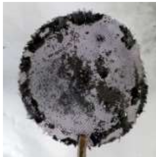
(a) Trapped biochar from 1 kg at 400 °C (b) Trapped biochar from 1 kg at 500 °C
