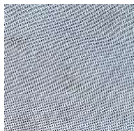
Figure 5: Stainless steel test wire mesh for trapping the biochar
