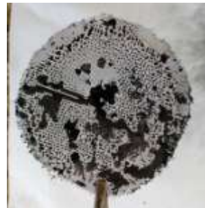
(c) Bio oil-stained sieve for 2 kg at 200 °C (d) Bio oil-stained sieve for 2 kg at 300 °C
