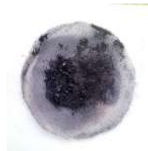
(a) Trapped biochar from 1 kg at 400 °C (b) Trapped biochar from 1 kg at 500 °C
