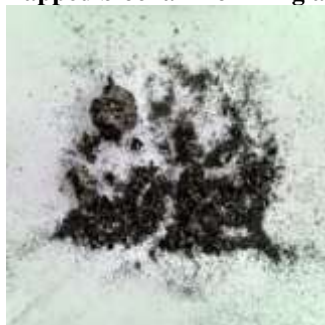
(a) Trapped biochar from 3 kg at 400 °C
