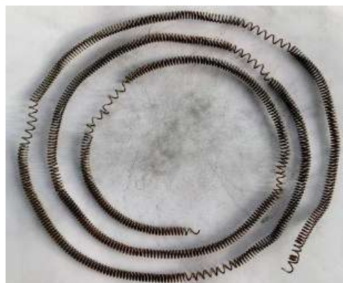
Plate 6: Heating element of the reviewed reactor for pyrolysis process before use
