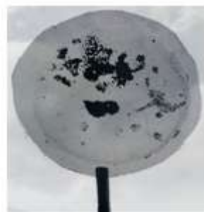
(a) Bio oil-stained sieve for 1 kg at 200 °C (b) Bio oil-stained sieve for 1 kg at 300 °C
