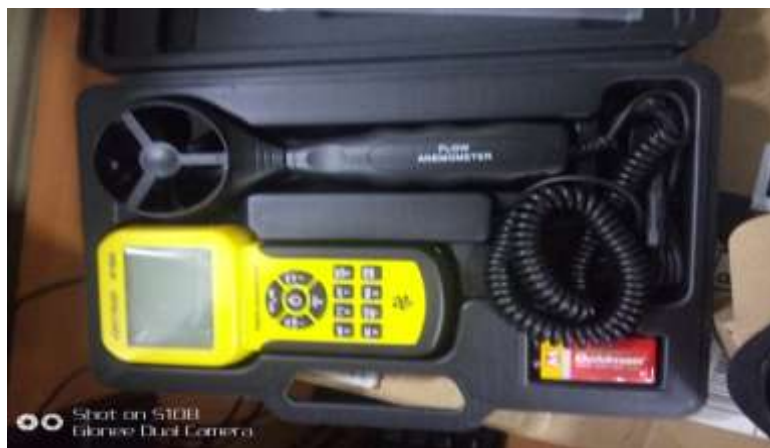
Fig. 9: An Anemometer for Measuring Air flow of ACs
