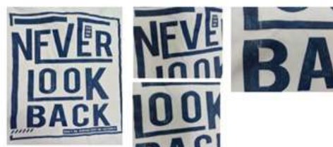
Figure 26. Water-based ink after 18 washes
