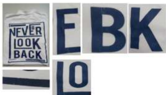
Figure 22. Water-based ink after 5 washes
