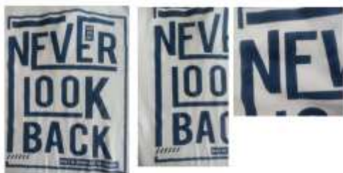
Figure 24. Water-based ink after 10 washes
