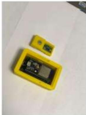
Fig.10 MAX3100 sensor with ESP32
