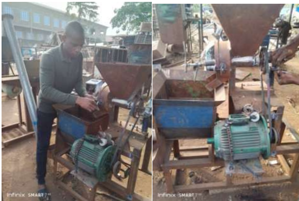
Figure 3.4 Picture of the milling-mixing machine during assembly for testing
