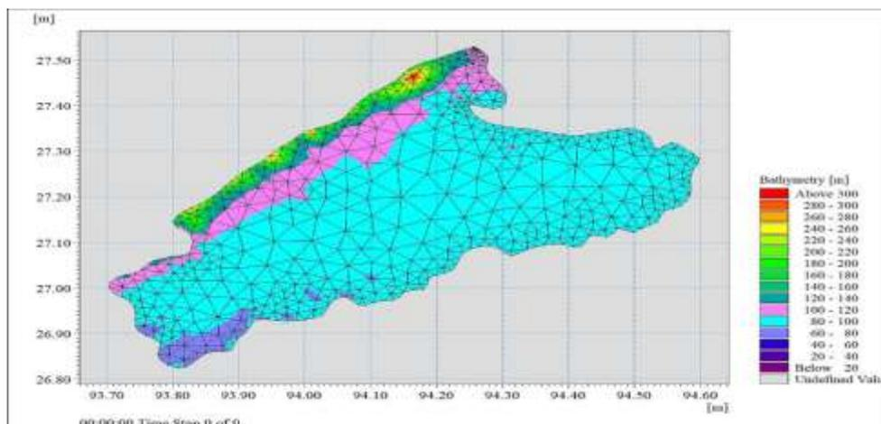
Figure 5.7: Resulting mesh bathymetry
