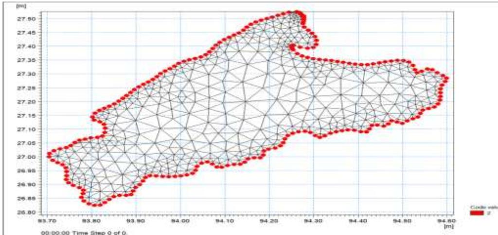
Figure 5.6: Resulting mesh after smoothing 100 times
