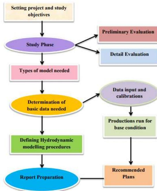
Figure 3.1: Flow chart of Flood Modelling
