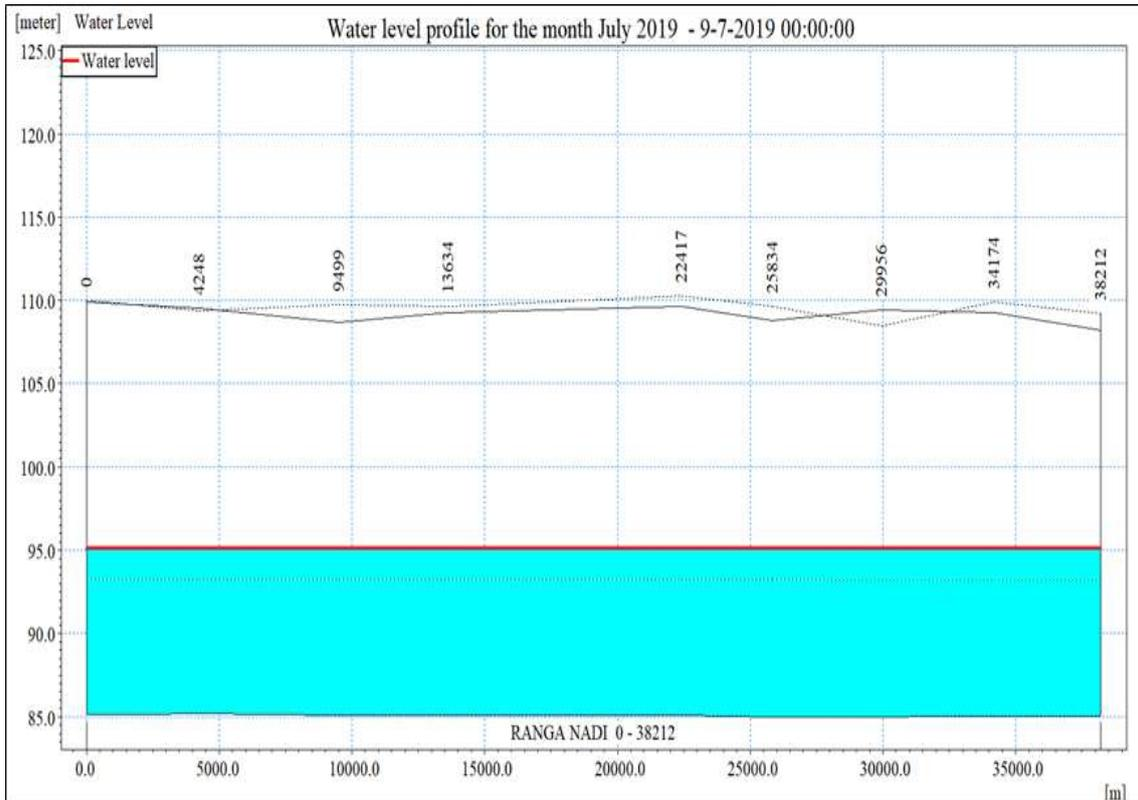
Figure 6.2: Longitudinal water level profile for the month July 2019
