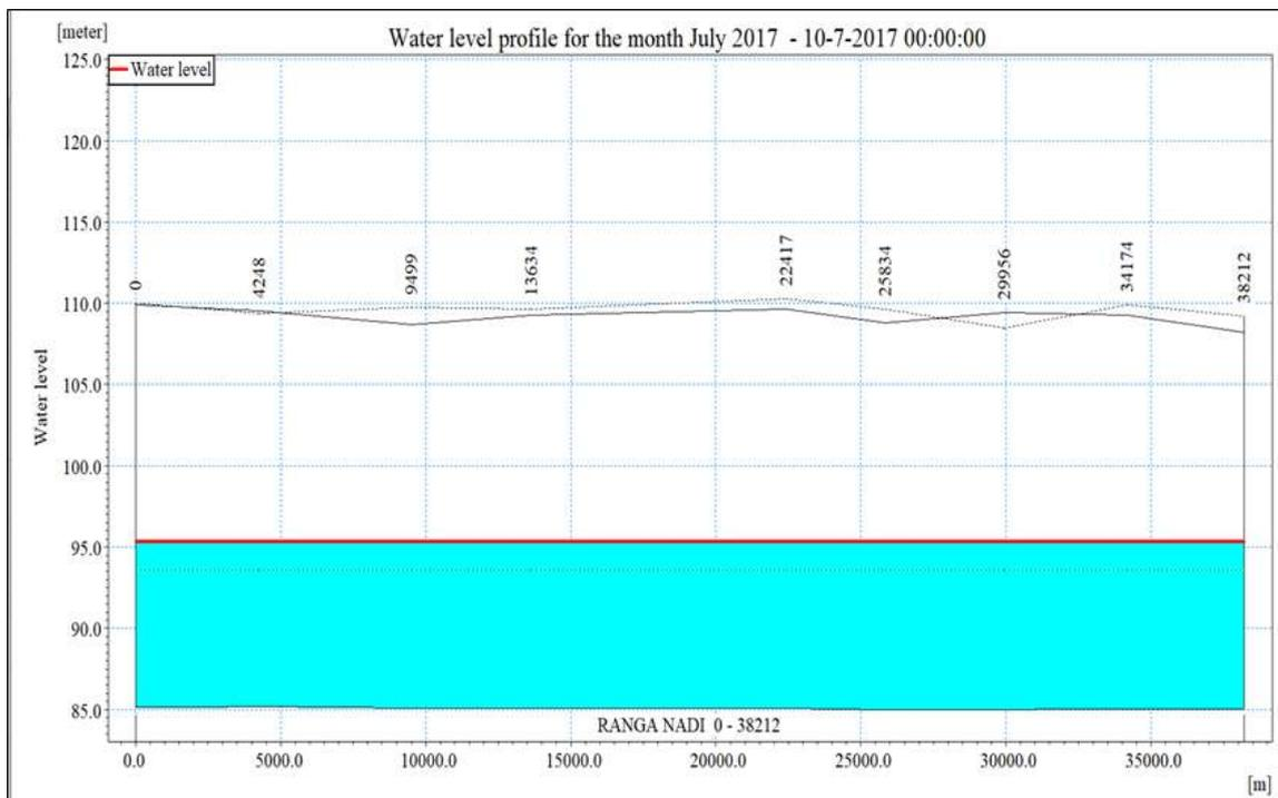
Figure 6.1 : Longitudinal water level profile for the month July 2017
