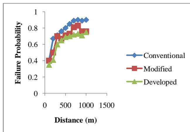
Fig.20: Probability of false handoff initiation for the various algorithms
