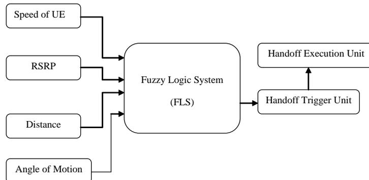
Fig.9 Architecture of FLS
