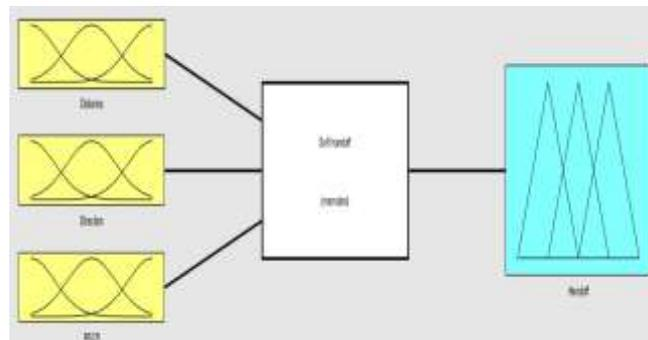
Fig.12 The FIS model for a system that limits its performance metrics to distance, direction and RSRP
