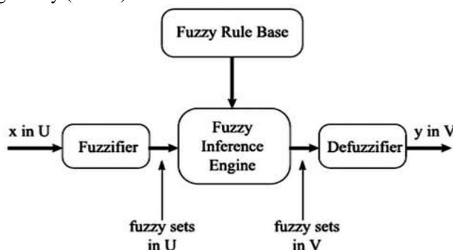
Fig.3 A Generalized Example of Fuzzy Logic System [13].
