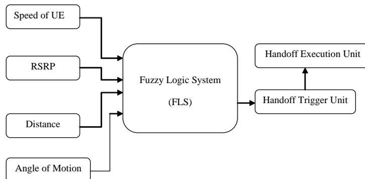
Fig.9 Architecture of FLS
