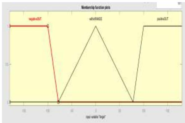
Fig.5 Angle of motion membership function
