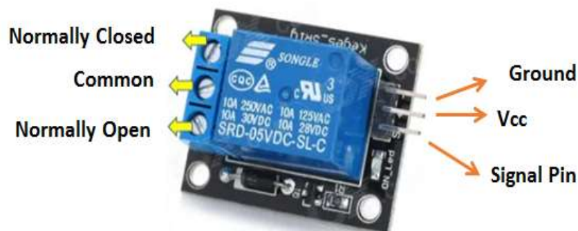
Fig-6 RELAY CIRCUIT.
