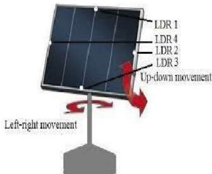
Fig. Schematic diagram Dual Axis Solar Tracking System
