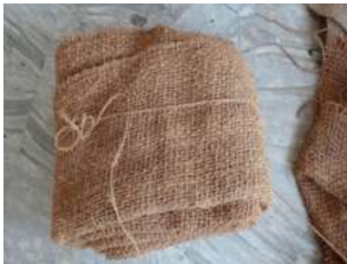
Fig-1: Unmodified coir geotextile
