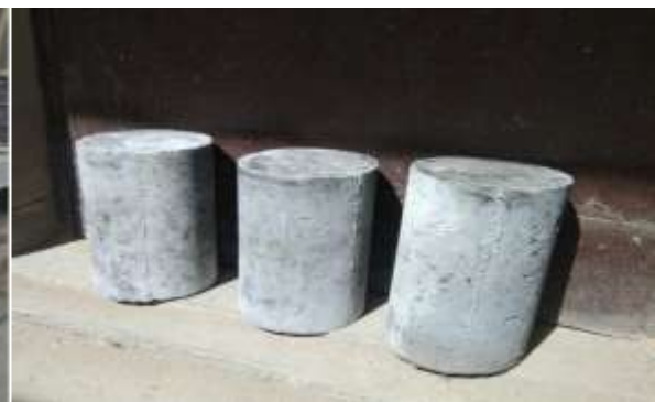
(b) Casting Cylinder Sample
