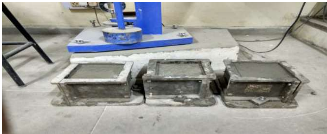
Figure 3.2:-Casting Cube Sample
