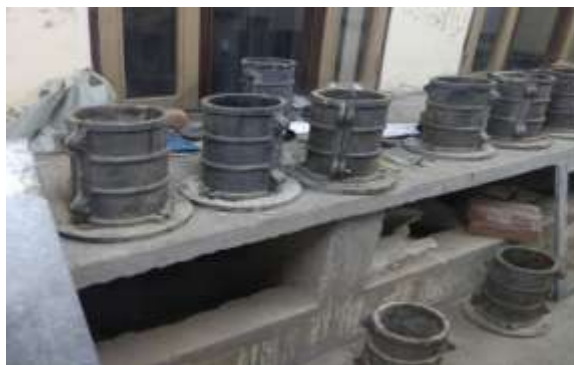
Figure 3.3:- (a) Cylinder Mould
