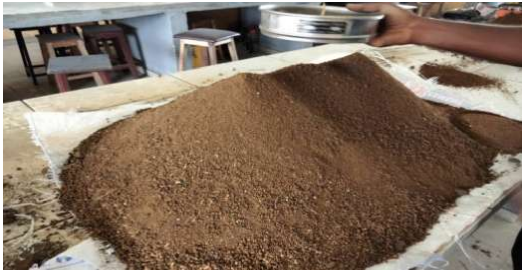
Fig.1. Prepared lateritic soil
