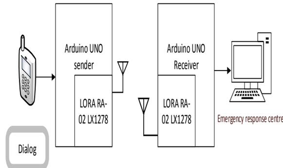
Fig.1 Signal Transmission through LoRa module
