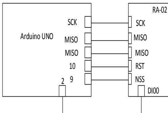
Fig. 4. Circuit connection of Arduino UNO with LoRA module
