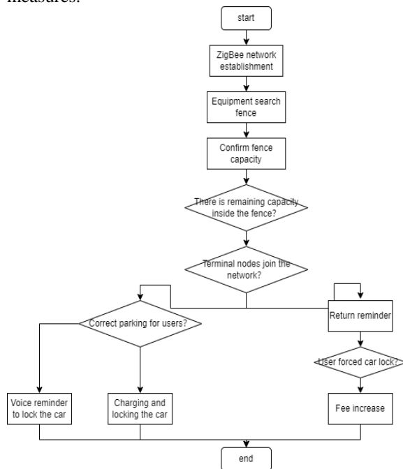
Fig.4. Workflow of electronic fence system
