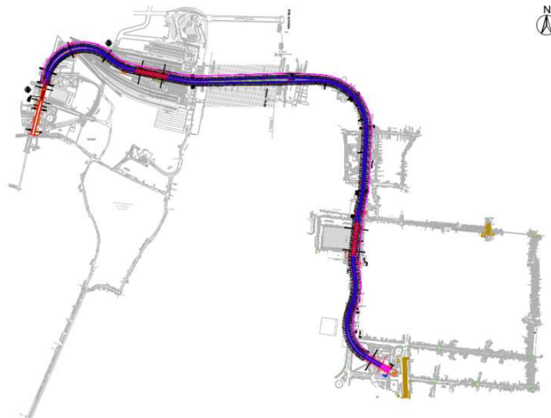
Figure.1 Kolkata East West Metro UG1 Tunnel Alignment
