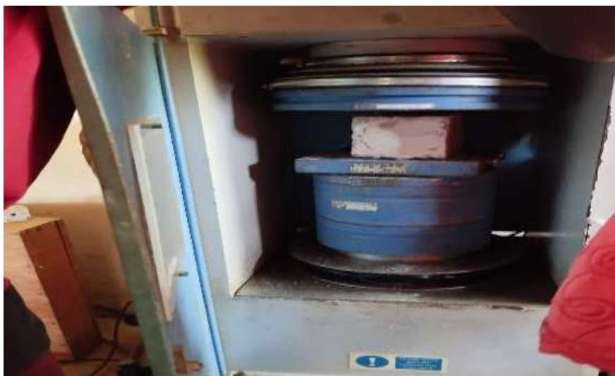
Figure 1: Testing Machine Compressive Strength Set up
