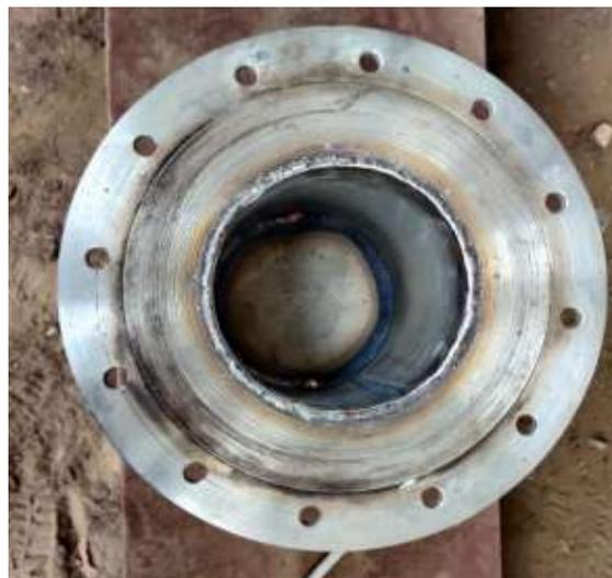
**(Top view of fabricated reactor)**
