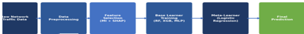
Figure 1. EnsembleShield++ End-to-End Pipeline: Raw Traffic → Preprocessing (SMOTE-ENN) → Feature Selection (MI + SHAP) → Base Learner Training → Meta-Learner → Final Prediction.
