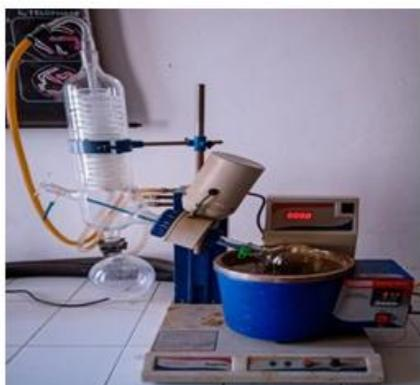
(Fig: 3 ) Rotary evaporator
