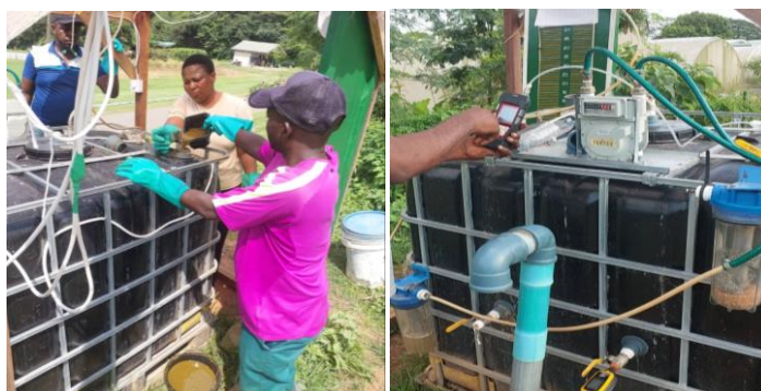
Figure 1. Loading process of cow dung slurry into bio-digester
