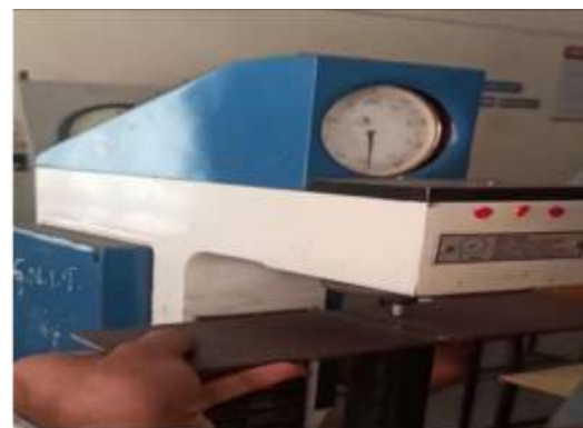
Hardness test conducting on Hardness testing machine
