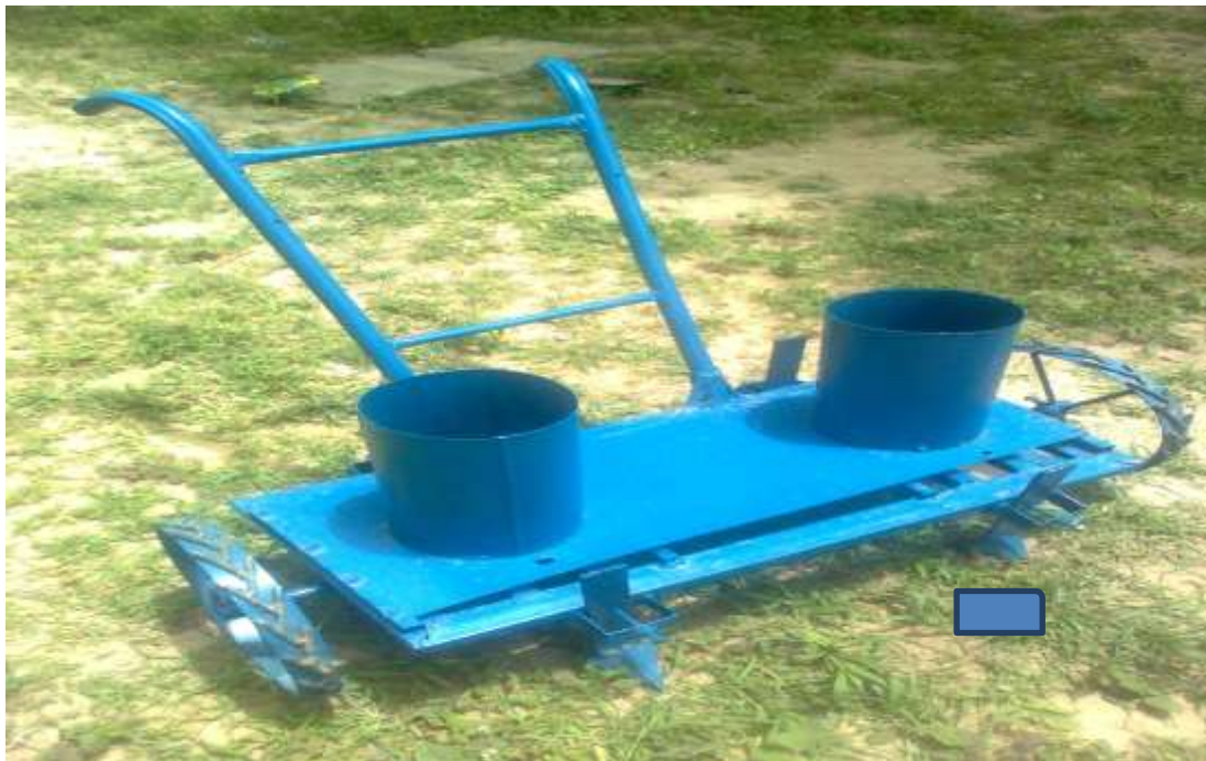
Figure2. The combined (maize and soya bean) seeds mobile planter
