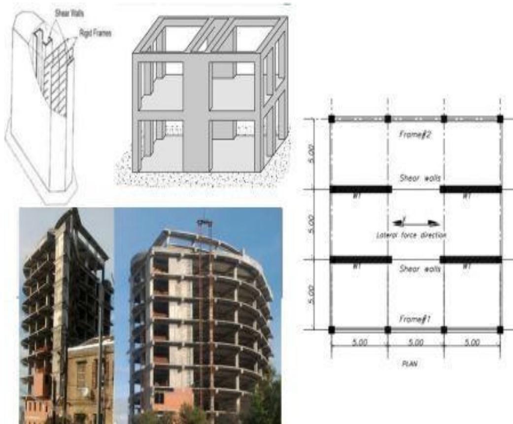
Fig.5) Wall Frame structural system (Dual system)
