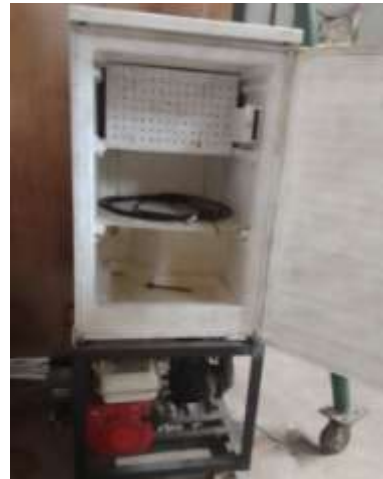
Figure 3: Assemblage of Gasoline-driven Refrigeration System
