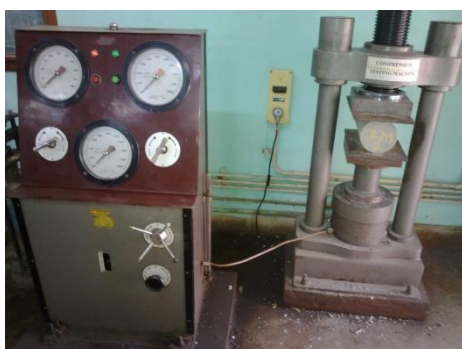
Figure 4.2 Split Tensile Test on Concrete Cylinder
