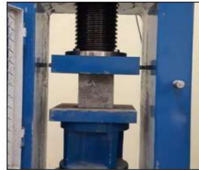
Fig. 1 Testing of cube
