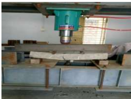
Fig. 8 Failure pattern of CB
