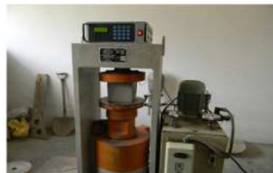
Fig 3.14: Experimental Setup For Testing of blocks Specimen by Digitally
