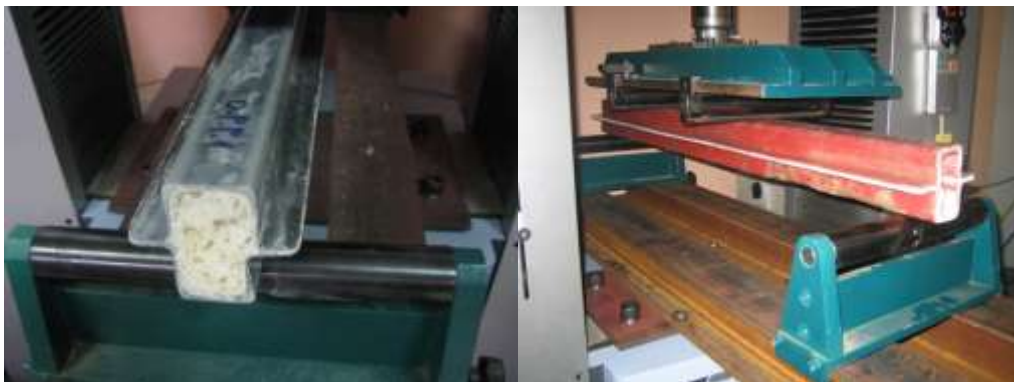
Figure 9. Testing of GFRP with and without PUF
