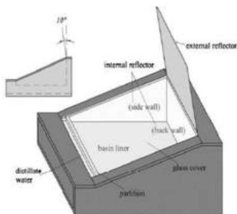
Fig No 01 Solar still with external mirror
