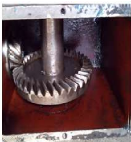
Plate 4: Interior view of Reverse-gearbox assembly consisting of pinion, ring gear and shaft
