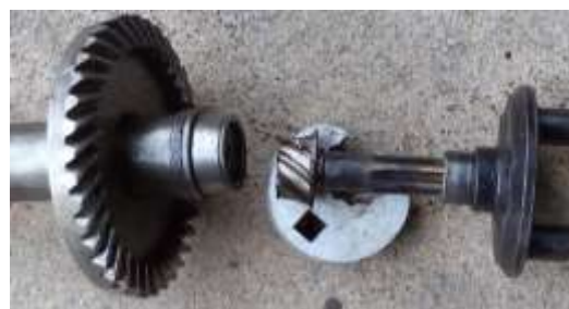
Figure 3: Failed components (from L-R): Ring gear and shaft, pinion, coupling, and rubber-damper
