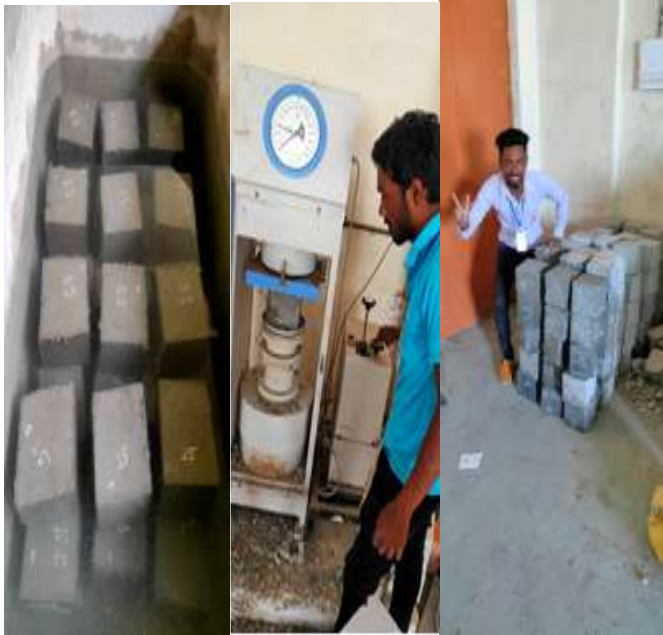
Fig: Cubes kept in water curing tank, testing of cubes by using Compressive testing m/c, Completion of project work.
