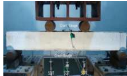
Figure 3. Test setting and four-point loading configuration
