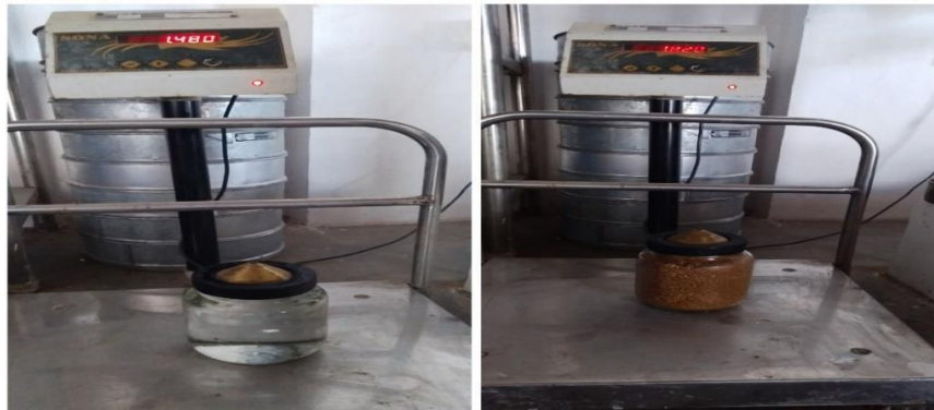
Fig.3.3 Specific gravity of fine aggregate
