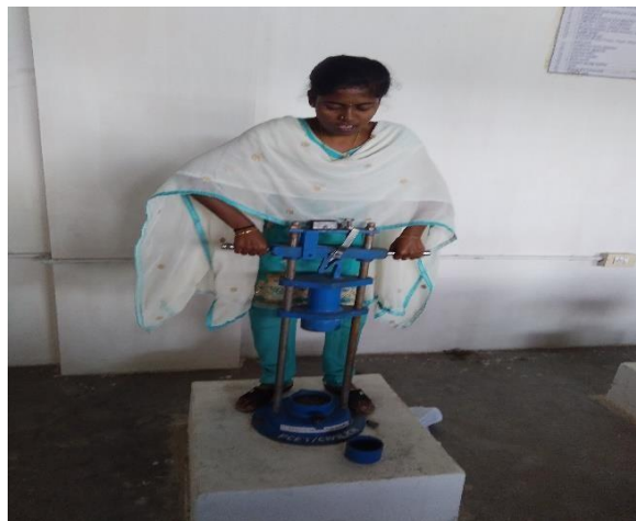
Fig .3.4 Impact test on Coarse Aggregate
