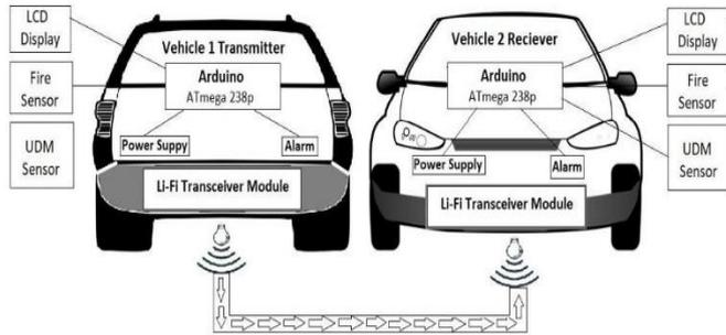
Figure 1.1. Block diagram of V2V communication using Li-Fi technology
