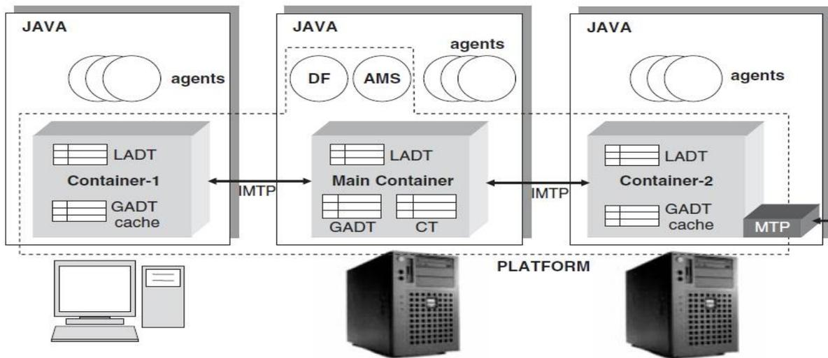
Fig. 6: Architectural elements of the multi agent based platform [4]
