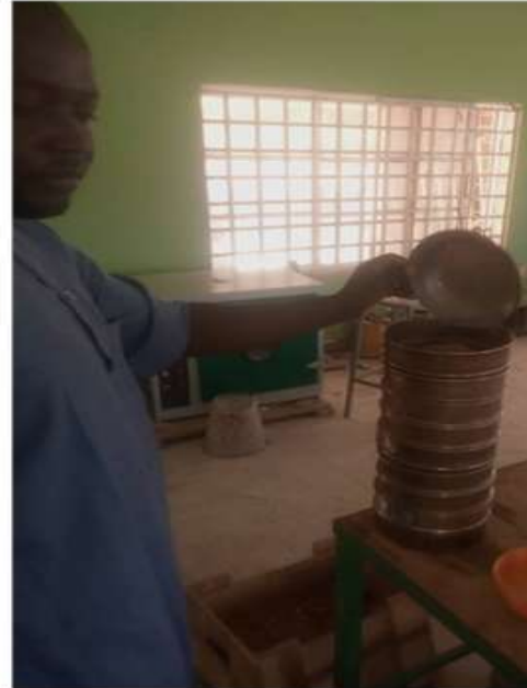
Fig. Performing Sieve Analysis for fine aggregate
