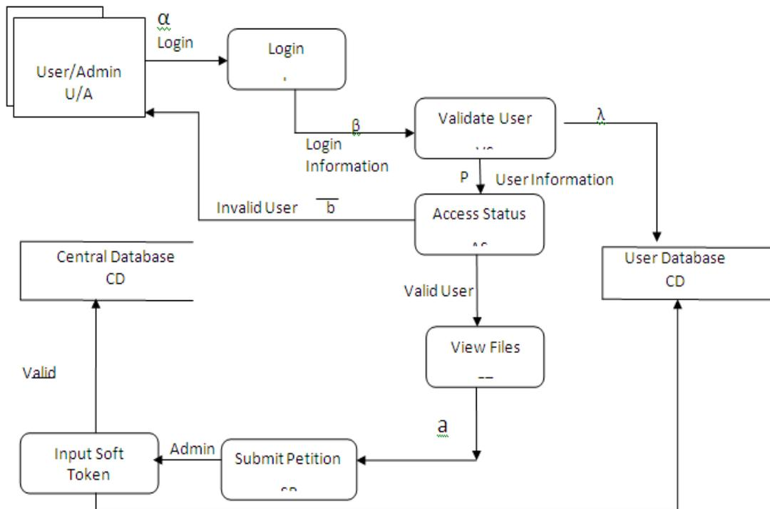
Figure 3.6: Data Flow Diagram of the New System Model, Source Field Work (2021)
