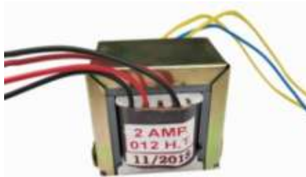
Fig.14:Step up Transformer.
