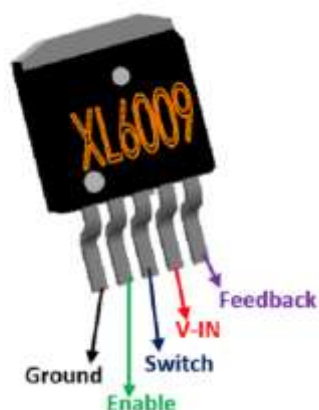
Fig.10:XL6009 Switching Regulator
