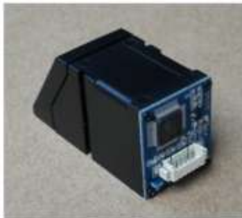
Fig 2: Back view of fingerprint module used (R305)
