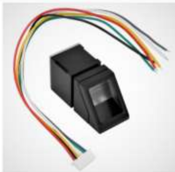
fig 1: front view of fingerprint module used. (R307)
