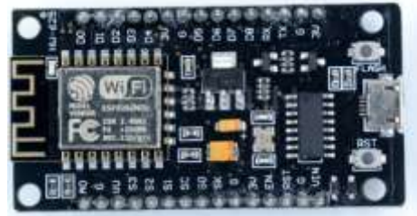
Fig 3: Nodemcu used for our project.
