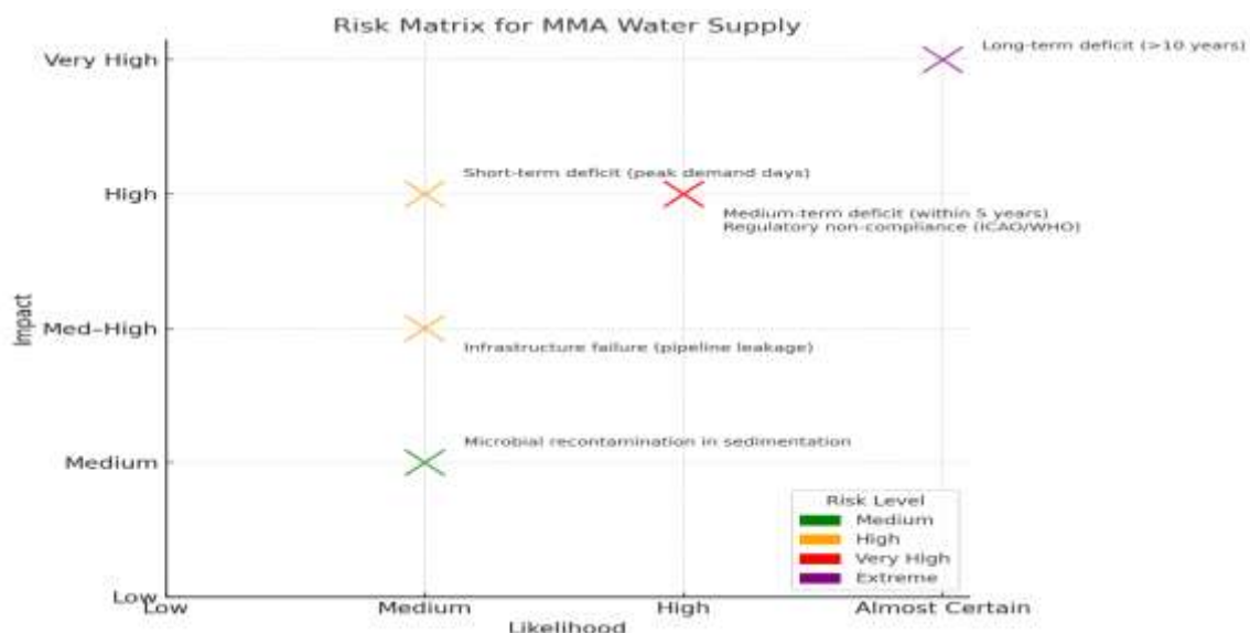
Figure 3.4: Colour-coded risk matrix for MMA water supply showing likelihood–impact positioning. Long-term deficits are extreme, medium-term deficits and regulatory non-compliance are very high, while short-term deficits and pipeline leakage are high risks.
