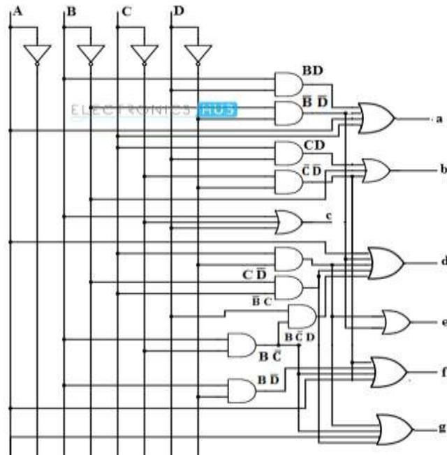
Figure 3 Gate level design of BCD to 7 Segment Display
