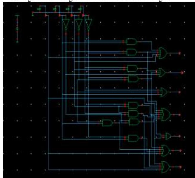
**Figure 7 Designed decoder circuit**
