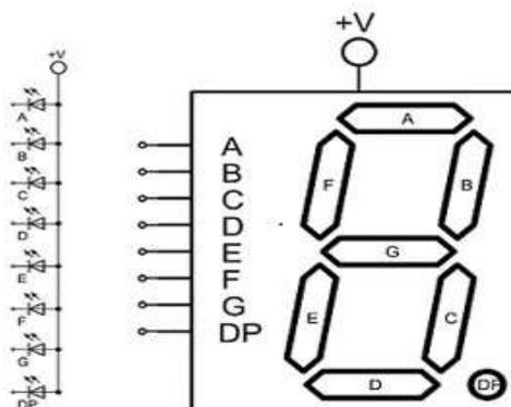
Figure 1 Seven segment common anode display
