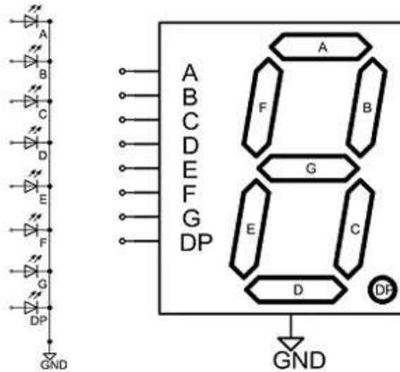
Figure 2 Seven segment common cathode display
