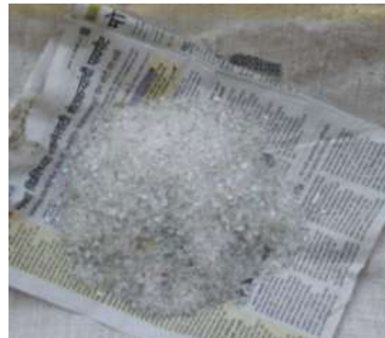
Fig.: Crushed glass for replacement as sand.
