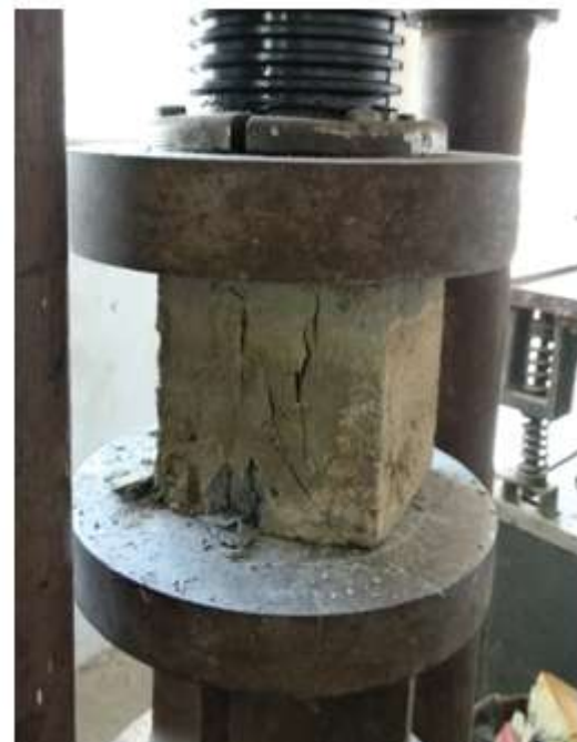
Fig.: failure of block due to compression.
