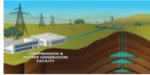
Compressed air energy storage
