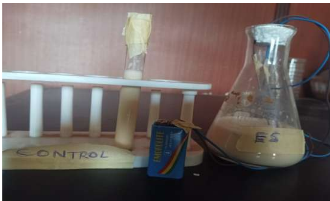
Figure 1: Setting-up circuit for electrical stimulation of milk
