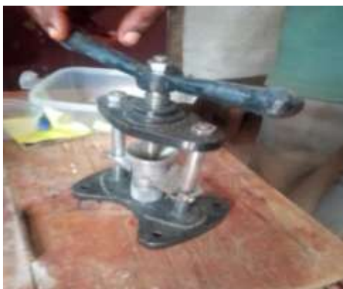
Figure 2.2 pelletizing combination of various proportions of coconut shell and coal
