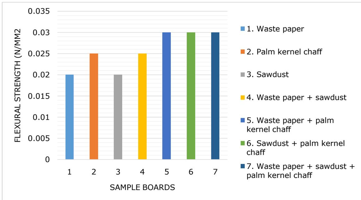
Figure 3: Flexural Strength Test
