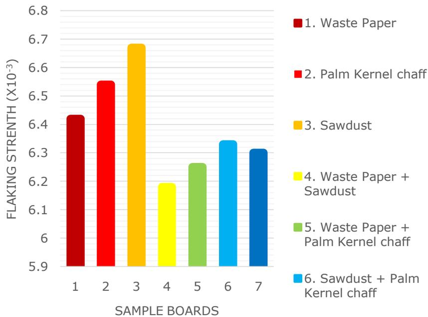
Figure 2: Flaking Test of the Boards
