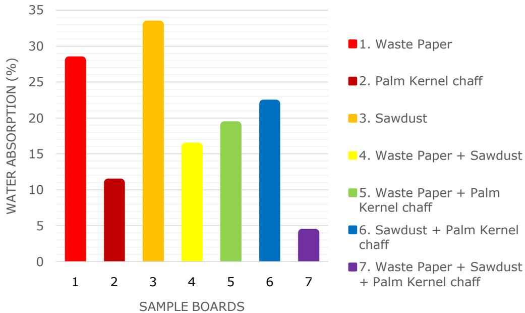
Figure 1: Water Absorption Percentage of Sample Boards
