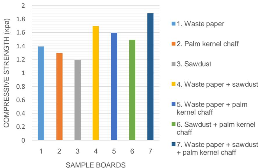
Figure 4: compressive Strength Test
